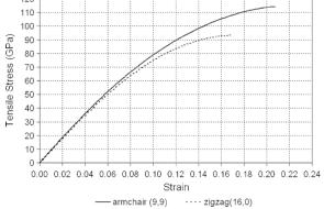
Comparison of two types pf carbon nanotubes in term of tensile stress and strain.
