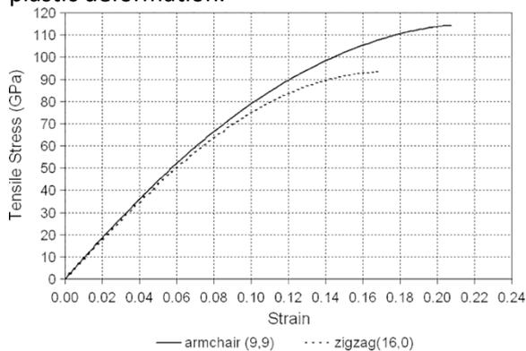
Comparison of two types of carbon nanotubes in terms of tensile stress and strain.
